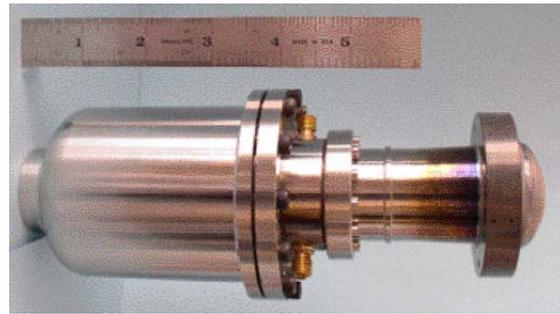
*Figure 4. NASA/Sunpower Advanced Stirling Generator unit, containing a Stirling engine and linear alternator. Two such units are used in an "ASRG".*
