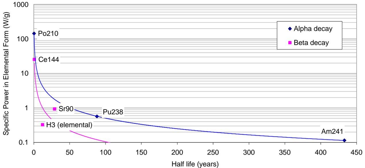
Figure 2. Isotope Specific Power as a Function of Half Life.
