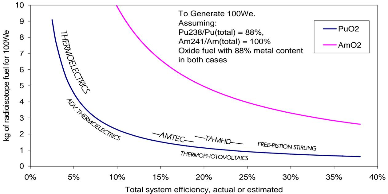
Figure 3. Isotopic fuel requirement vs. converter system efficiency.
